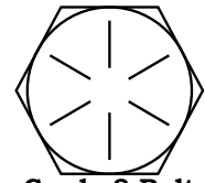
Grade 8 Bolt Head Marking
