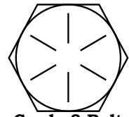
Grade 8 Bolt Head Marking
