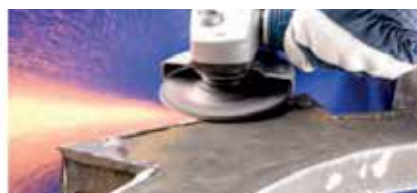
Rough grinding & weld removal
