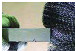
INCORRECT Excessive pressure can cause wire breakage
