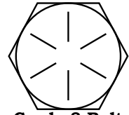
Grade 8 Bolt Head Marking
