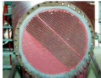
Tube sheet repair performed for Carrier Corporation.
