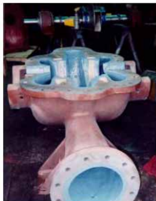
ML406 BRUSHABLE CERAMIC - River Discharge Pump - Inland Container, Orange, TX
