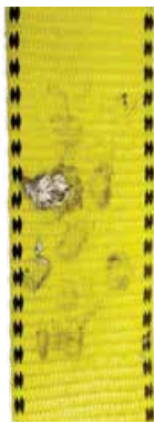
SLING WELDING SPLATTERS
