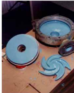
ML406 BRUSHABLE CERAMIC - Centrifugal Pump Coating - Temple Inland, Buna, TX
