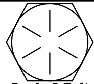
Grade 8 Bolt Head Marking
