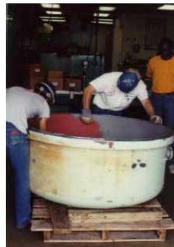
ML406 BRUSHABLE CERAMIC - River Discharge Pump - Inland Container, Orange, TX
