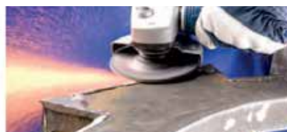
Rough grinding & weld removal
