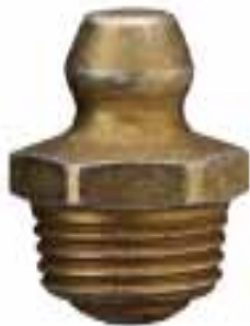
1/8" Pipe Special Taper Thread Rec. Hole Size - .373 to .380"
