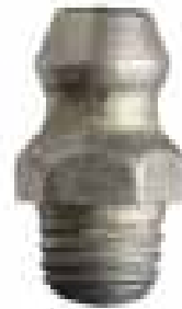
1/4"-28 Special Taper Thread Rec. Hole Size - .230 to .235"
